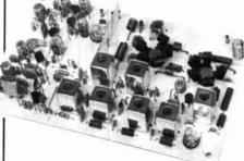
T51 VHF FM EXCITER for 10M, 6M, 2M, 220 MHz or adjacent bands. 2 Watts continuous, up to 21/2 W intermittent. \$68/kit.
